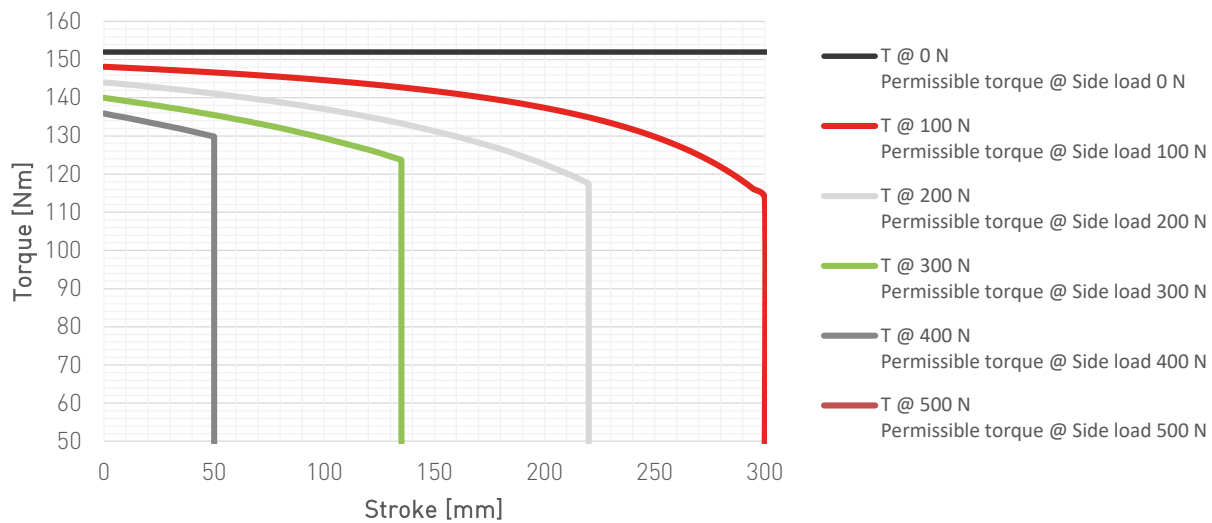
Permissible torque for a given side load EA015 - stroke 250 mm
